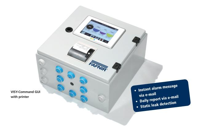
VISY-Command GUI contains the intrinsically safe power supply for the VISY-Stick sensors and their control unit. Various interfaces ensure that it always has access to the latest data. The integrated display unit with the 5.7" colour touch screen provides and displays the current measurement values and the reporting functions (log file) in a user-friendly form.
